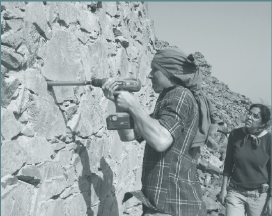
From left to right: Jack Johnson (UW) and Margaret Brown Enrile (Illinois-Chicago) collecting a mortar sample for luminescence dating from ancient fortifications at Acaray, Peru; Julie Brugger thinking about the relationship between landscape and democracy while looking out over the Escalante desert in Utah; Andrea Duncan with a one-year-old male orphaned orangutan at the rescue and rehabilitation center at Taman Safari, Bogor, West Java, Indonesia.
